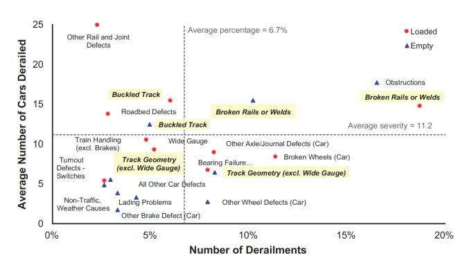
Li, W., Roscoe, G.S., Zhang, Z., Saat, M.R. and Barkan, C.P., 2018. Quantitative analysis of the derailment characteristics of loaded and empty unit trains. *Transportation Research Record*, 2672(10), pp.156-165.
